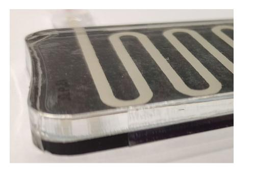
The heating systems were sandwiched between two polymeric pieces, with the front one having **different thicknesses** (5 mm and 3 mm).
